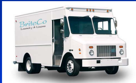
Workhorse W42 Chassis step-van chassis w GM 4.8L engine, and Workhorse W62 with GM 6.0L engine; FCCC MT45 chassis with GM 6.0L (soon)
