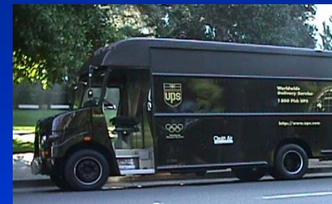
Workhorse W42 Chassis step-van chassis w GM 4.8L engine, and Workhorse W62 with GM 6.0L engine; FCCC MT45 chassis with GM 6.0L (soon)
